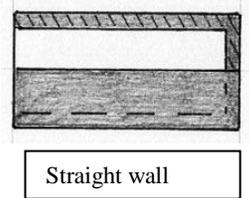
Most pistol jackets will be straight walled jackets. Usually handgun jackets will be short compared to a rifle jacket and the pistol ogives used are fairly blunt and in this case the straight walled jacket works quite well.
