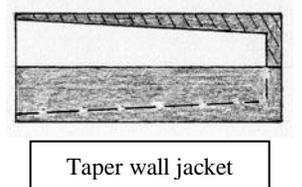
For rifle calibers up to about .257 the jacket is usually made with a uniform taper running from the base of the jacket to the mouth of the jacket. This taper is not large being between 1/3 of a degree per side to perhaps 2 degrees per side. If the angle is too large there will be a tendency for the core to pop back out of the jacket once the core has been seated and it will make it harder to fit the seating punch to the jacket.
