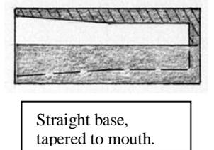
A variation on the straight wall/tapered jacket has the jacket taper from the base to part way up the jacket. Then the jacket has a thinner straight
