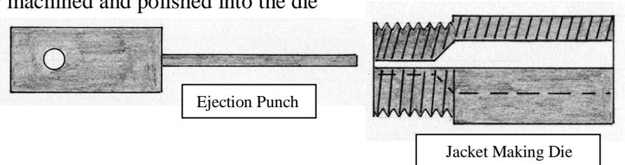
The piece of tubing that will become the jacket is pushed into the die by a *jacket making punch*. The punch has a tip that fits down into the tube and is a snug fit to the tube. There is a collar on the punch that will push against the mouth of the tube. The tip of the punch supports the tube to keep it from buckling or collapsing as it is pushed into the die. A jacket making set will include three and possibly more forming punches. Each punch makes one length of jacket.
