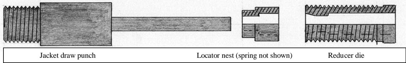
ram. The punch may have a locating nest on the punch that will help to keep the jacket square to the die as the jacket enters the die. The locating nest has a compression spring that holds the nest up and keeps a little pressure on the jacket.
