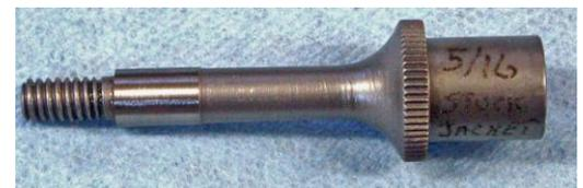
Stuck Tube Removal Punch
